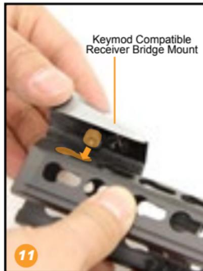
11. On the Keymod Compatible Receiver Bridge Mount, hold the Keymod Nut in place and loosen the screw by turning it counter-clockwise with the included 3/32" Allen Wrench. Do not fully detach the Keymod Screw from the Keymod Nut.
