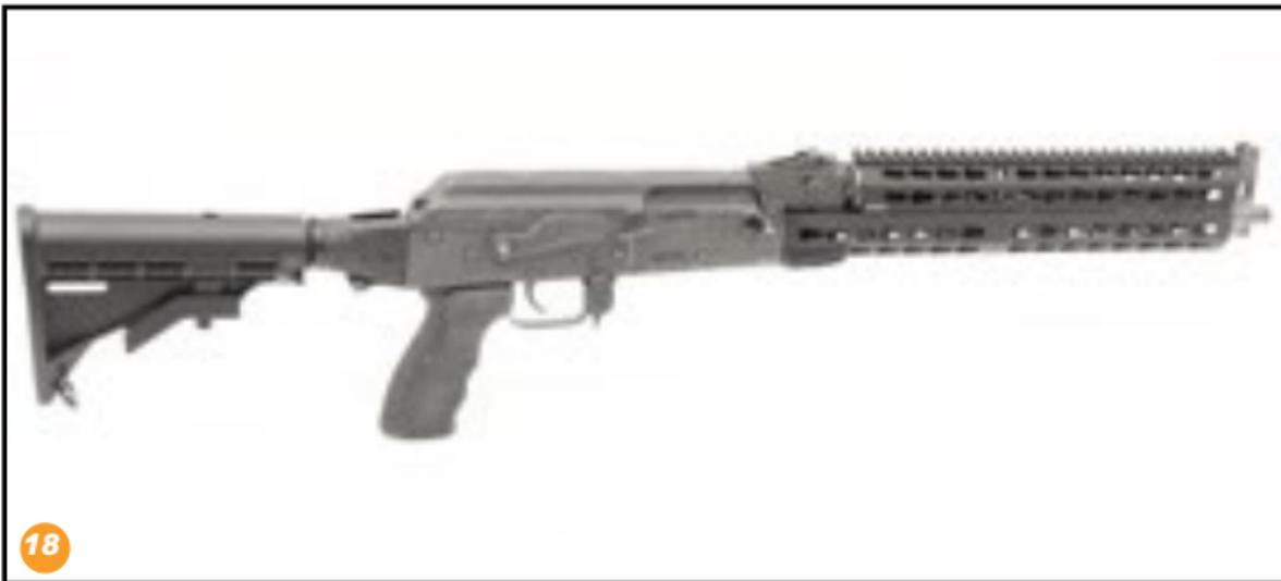
18. Replace the bolt, bolt carrier, action spring, retaining rod and the receiver cover according to your firearm owner's manual.
