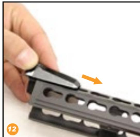
12. Place the Keymod Compatible Receiver Bridge Mount onto the last Keymod Slot of the lower handguard rail. Insert the nut through the larger portion of the Keymod slot. Ensure the protruding foot of the nut is pointing toward the muzzle of the firearm. Slide the Keymod Compatible Receiver Bridge Mount toward the muzzle until the mount fully drops into the handguard.
