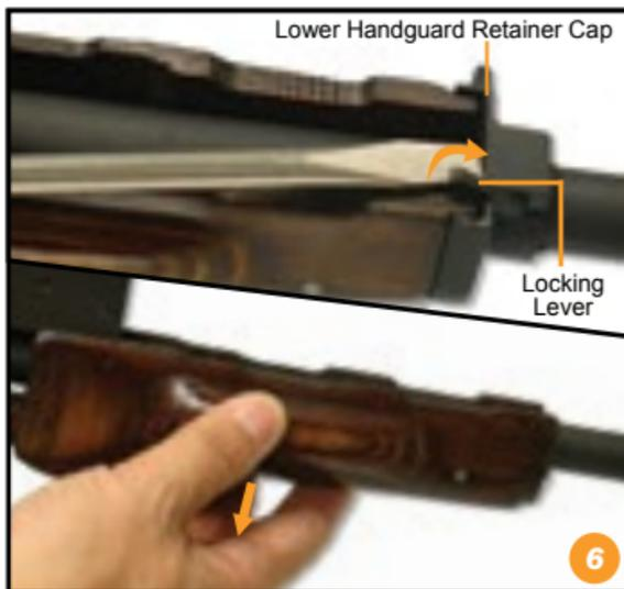
6. Unlock the Lower Handguard Retainer Cap by folding the Lever forward. Remove the Lower Handguard and leave the Handguard Retainer Cap unlocked for later assembly.
