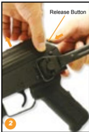
2. Press the Release Button to lift and remove the receiver cover.
