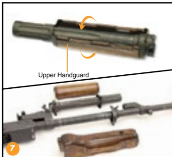
7. Twist the Upper Handguard to separate it from the gas tube. The gas tube will be reinstalled at a later time.
