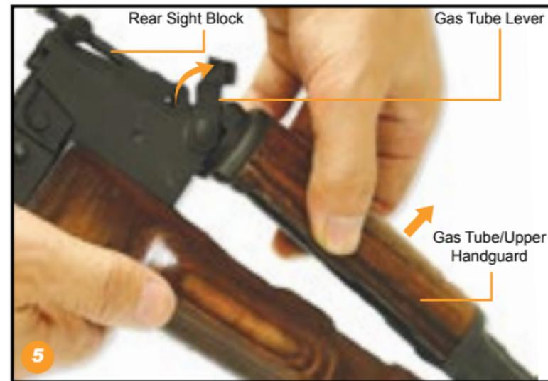
5. Lift and push forward the Gas Tube Lever next to the Rear Sight Block and take out the Gas Tube/Upper Handguard Assembly.
