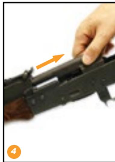
4. Remove the bolt and bolt carrier, including the gas piston attached to the bolt carrier.
