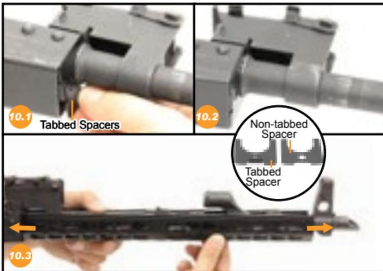
10. If forward and backward movement is detected, install the included Spacer(s) in the gap between the lower handguard and receiver.
