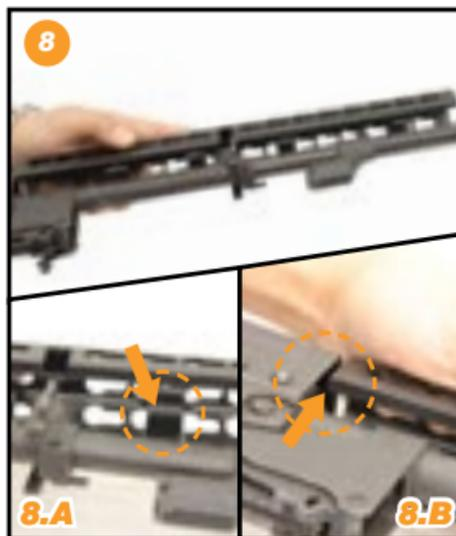
8. Perform a pre-installation check. Fit the lower handguard onto the barrel and check for vertical tilting, and forward and backward movement.
